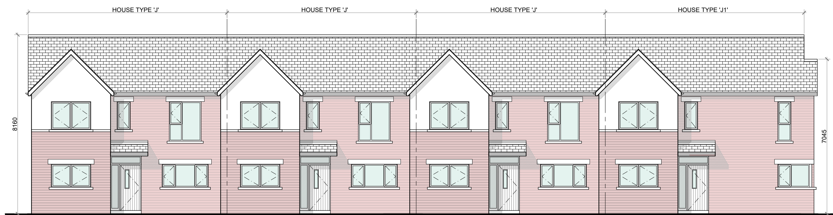
FRONT ELEVATION @ 1:100 TERRACE BLOCK TYPE 18
